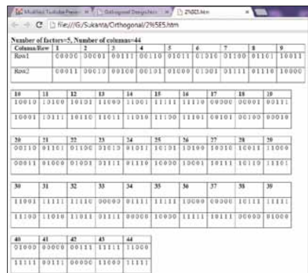
Row column design for 25 factorial experiment for orthogonal estimation of main effects and two factor interactions
